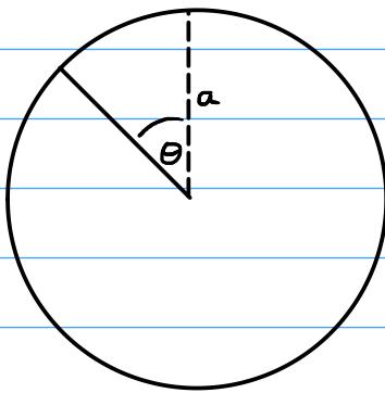
The vertical height above the centre of the wheel is  $a \cos \theta$ . The vertical component of velocity is  $a \omega \sin \theta$
